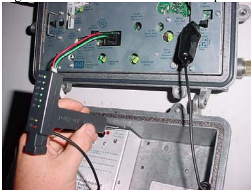
Fig. 1a: Power Clip™ inside trunk line amplifier
